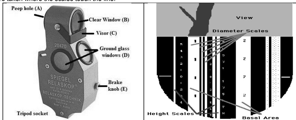
The Australian made Spiegel Relaskop contains the following scales from left to right: The 20 m height band, Band 1, The 4 narrow bands *i.e.* 2 white ones and 2 black ones in between, The 25 m height band. The 30 m height band, Band 2 and 7. The range finder bands Band 1 and 4 narrow bands are used for measuring tree diameter at any height on the tree stem.
