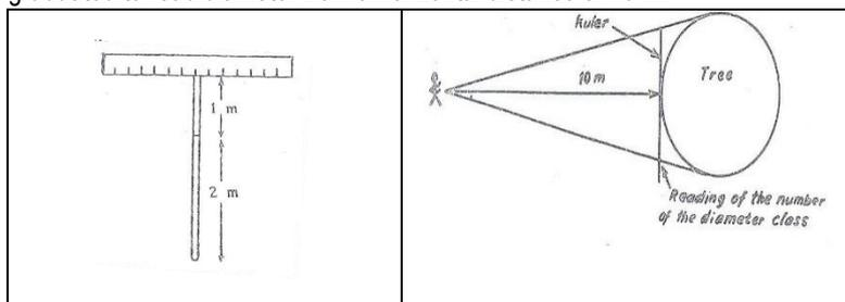
The ruler is usually graduated to read diameters from a horizontal distance of 10 m. In order to use the instrument, the observer stands at a horizontal distance of 10 m from the side of the tree. A helper places the ruler against the tree at the height of measurement, keeping it perpendicular to the line of sight and the left edge of the rule r in line with the left edge of 2 m the stem in relation to
